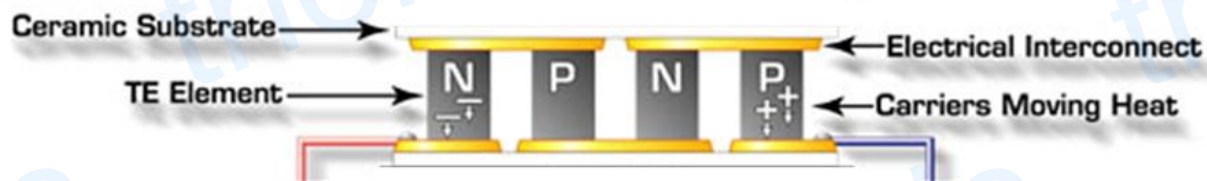
Figure 1 The structure of the Peltier modules
