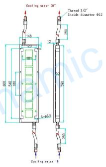
100 Watts Output Thermoelectric Power Generator Diagram
