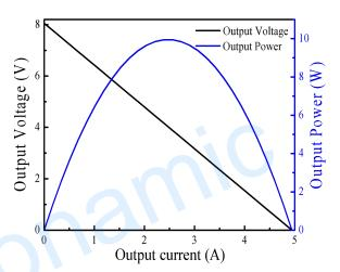
The chart for output voltage and output power Vs output current under  $T_h{=}300~^{\circ}C$  and  $T_c{=}30~^{\circ}C$
