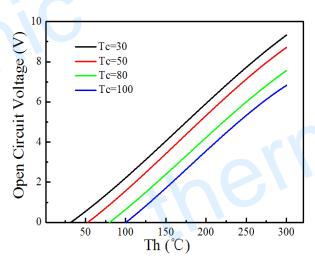
The chart for open circuit voltage Vs T<sub>h</sub> under various T<sub>c</sub>
