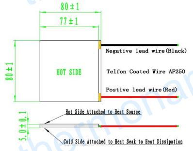
Note: The module clamping force should be in 700~800kgs.
