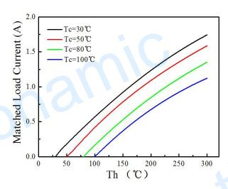
The chart for matched load current Vs T<sub>h</sub> under various T<sub>c</sub>
