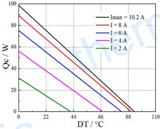
Performance Curves at  $T_h=50\text{ }^\circ\text{C}$
